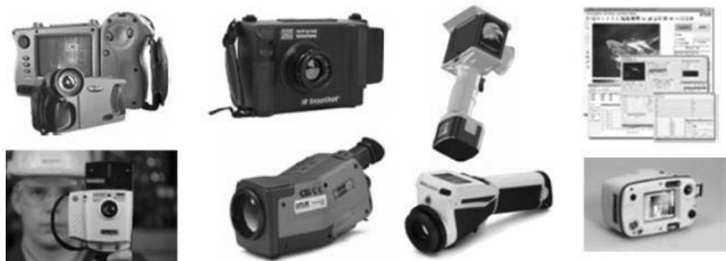
Figure A-20 Infrared Thermography instruments include Spot Radiometers, still cameras, and movie cameras.
