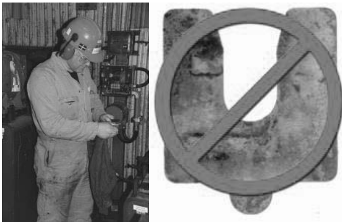
Figure 16-32 Clean shims and remove those that are rusted, bent or painted
