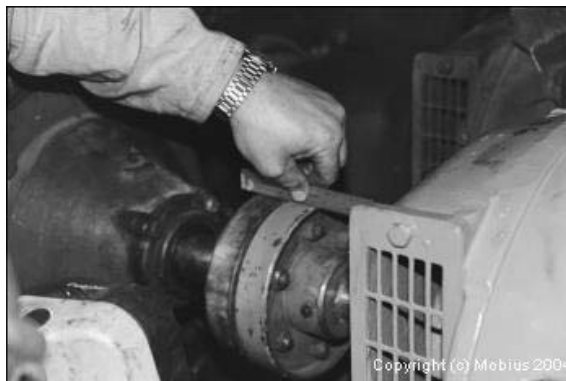
Figure 16-10 Machines will likely be misaligned if precision alignment was not performed
