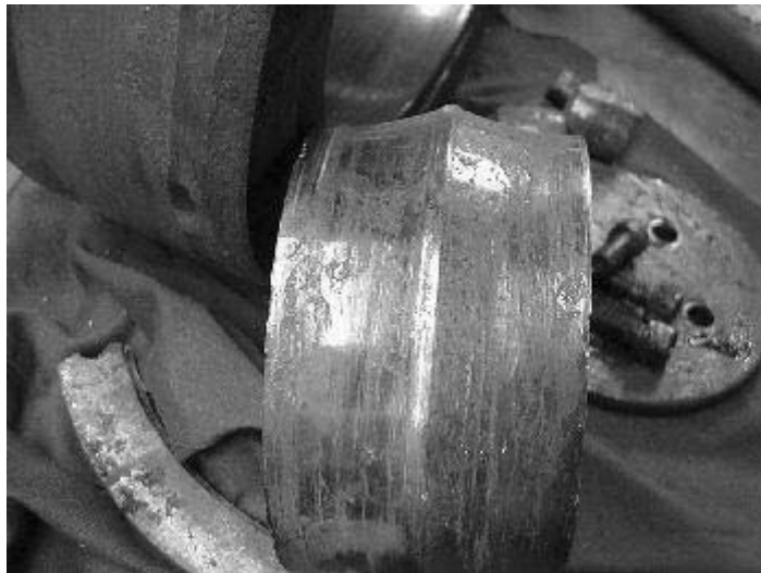
Figure B-12 Inner race bearing fault – why did this happen?
