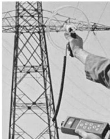
Figure A-10 A "dish" captures sound from a distance
