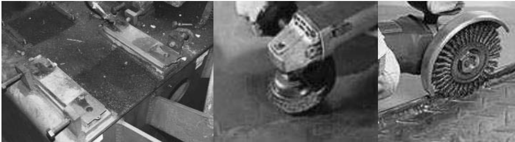
Figure 16-31 Remove dirt, grit, burrs and other debris
