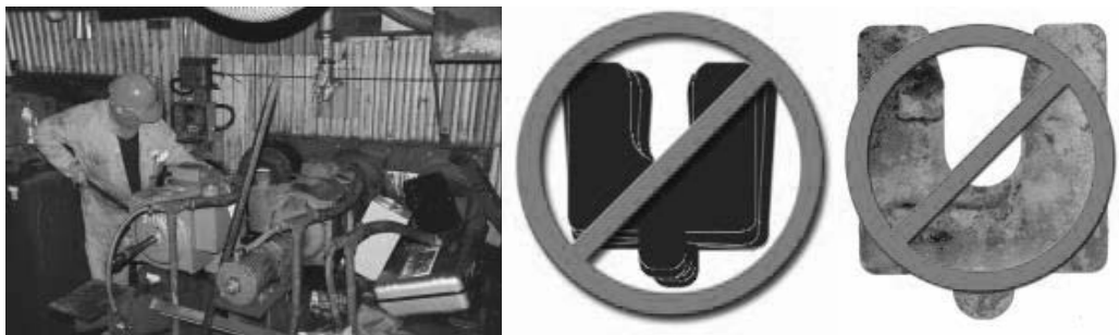
Figure 16-61 Using shims for vertical correction
