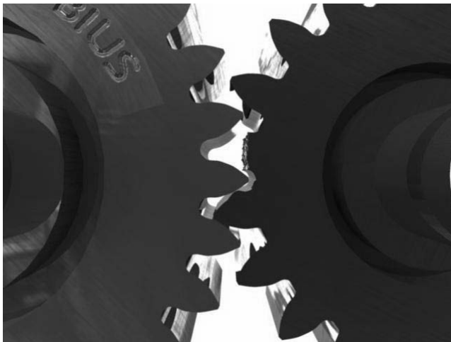
Figure 14-32 Gear with broken tooth
