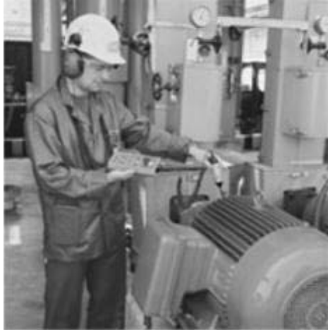
Figure A-16 Direct Contact probe is useful for detecting bearing problems
