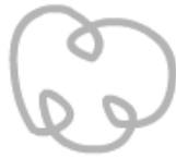
Figure 11-42 - Forward precession ( \frac{1}{3}X )
