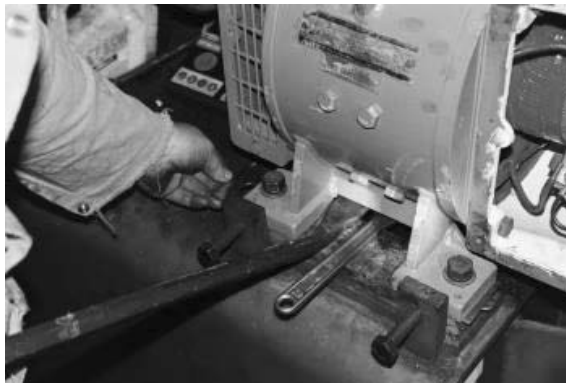
Figure 16-59 Adding a shim
