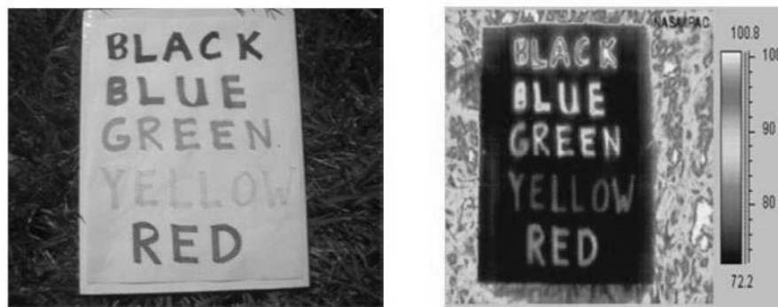
Figure A-25 The paper is all the same temperature. The color affects the Emissivity.
