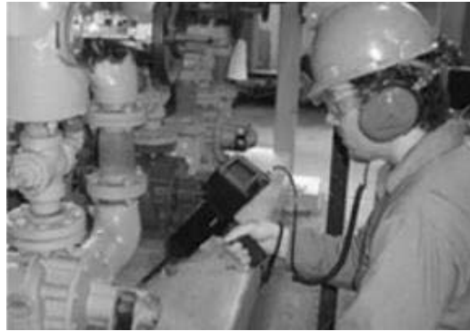
Figure A-11 A Direct Contact probe uses a “stinger” to capture the sounds
