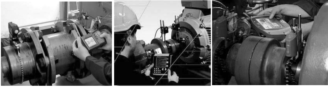
Figure 16-54 Modern laser alignment systems
