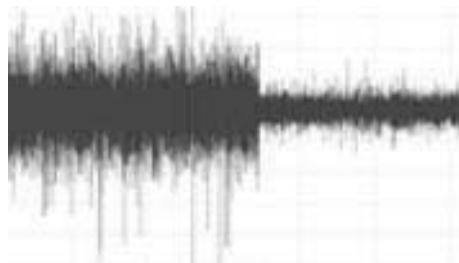
Figure A-18 Capture of Ultrasonic energy during lubrication
