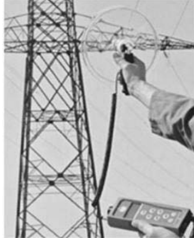
Figure A-15 Ultrasonics is a good choice for monitoring distribution lines
