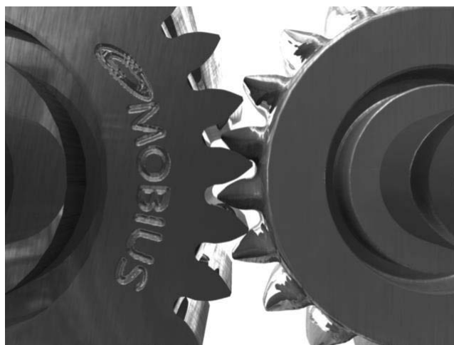
Figure 14-21 Very badly worn gear
