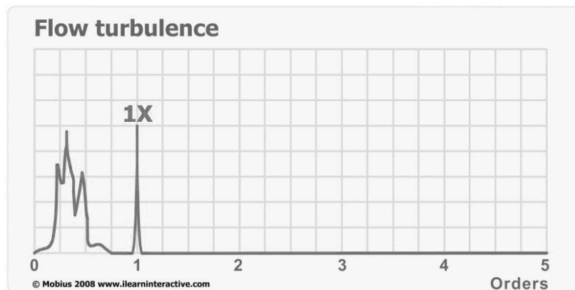
Figure 13-6 - Flow turbulence in fans and pumps
