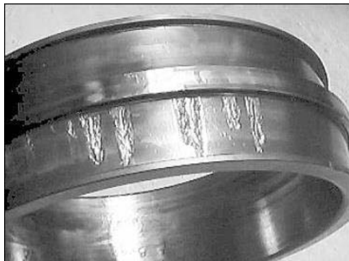
Figure 16-1 The majority of bearing failures are caused by misalignment
