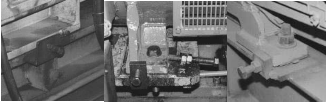
Figure 16-63 Jacking bolts for lateral movement
