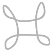
Figure 11-43 - Reverse precession ( \frac{1}{4}X )
