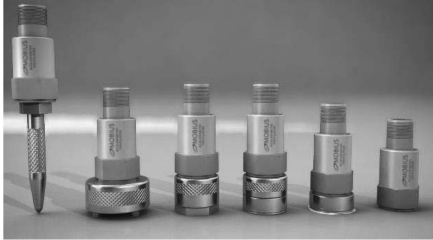
Figure 14-42 Accelerometer mounting options
