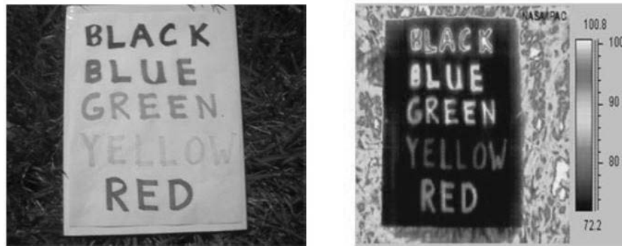
Figure 23-30 The paper is all the same temperature. The color affects the Emissivity.
