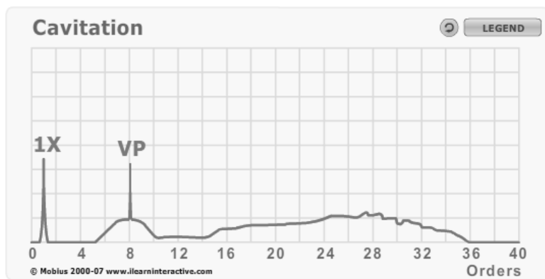
Figure 17-3 - Cavitation often has a hump of energy in the floor
