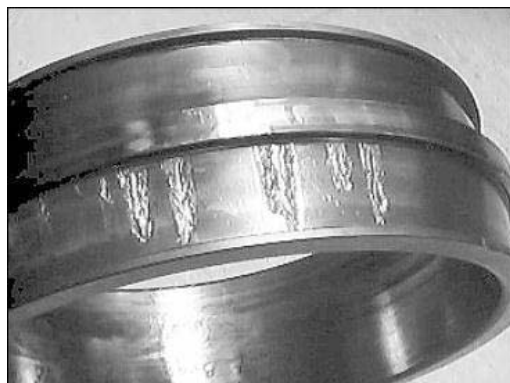
Figure 12-1 The majority of bearing failures are caused by misalignment
