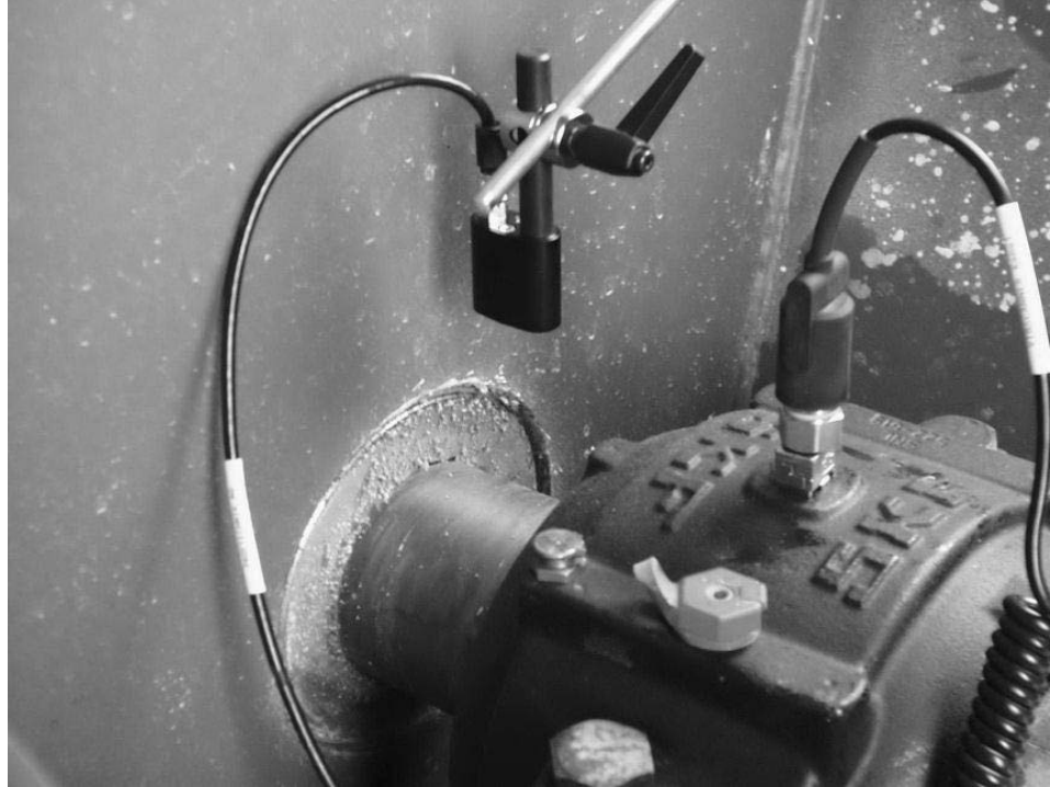
Figure 6-96 - A typical setup with laser tach and sensor
