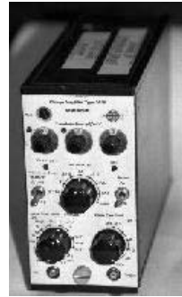
Figure 6-24 - Charge Mode amplifier for older style accelerometers.
