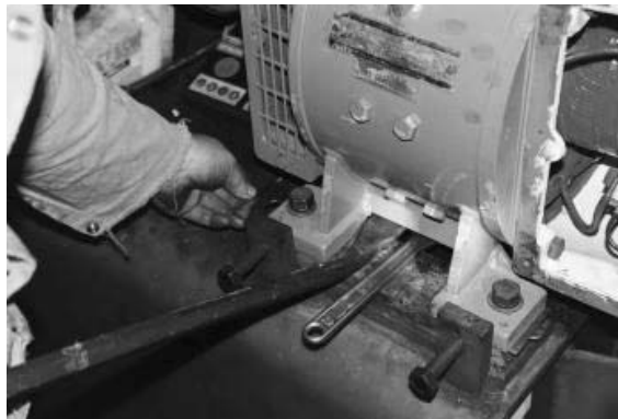
Figure 12-59 Adding a shim
