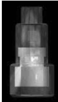
Figure 6-23 - crystal and mass in accelerometer
