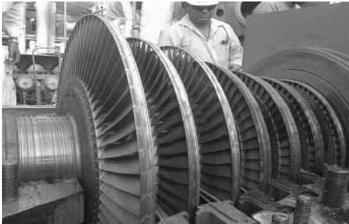
Figure 8-4 - Large, flexible rotors have Critical Speeds.
