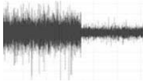
Figure 23-21 Capture of Ultrasonic energy during lubrication
