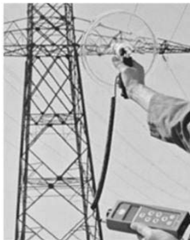
Figure 23-18 Ultrasonics is a good choice for monitoring distribution lines
