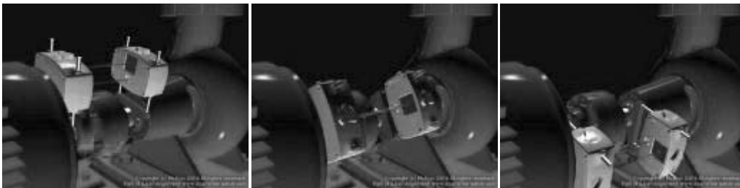
Figure 12-57 Gathering data through a 60 degree shaft rotation
