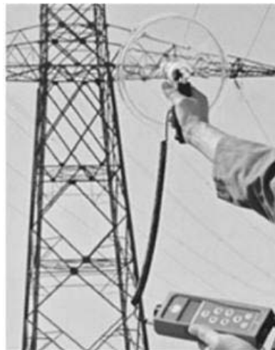
Figure 23-12 A "dish" captures sound from a distance
