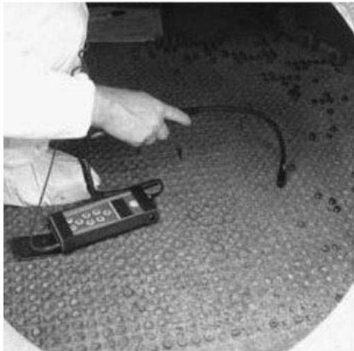
Figure 23-16 Sweep the microphone across the area to detect the leak.
