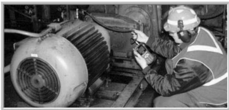
Figure 11-9 - Misalignment or Unbalance?
