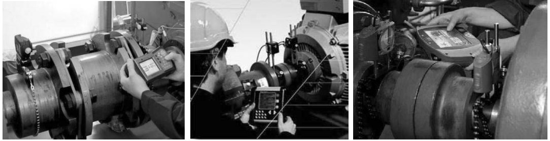
Figure 12-54 Modern laser alignment systems
