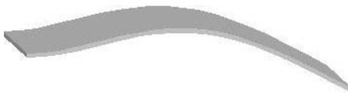
Figure 8-8 - Cantilevered bar bending in its second mode.
