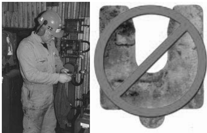
Figure 12-32 Clean shims and remove those that are rusted, bent or painted
