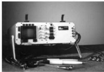
Figure 23-41 Baker Instrument used for Static tests
