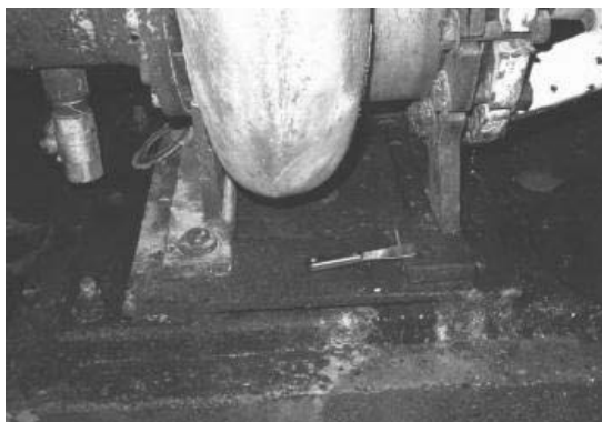
Figure 12-12 Misalignment can be detected via physical signs
