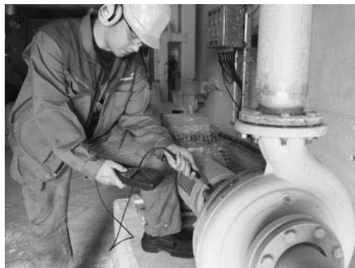
Figure 6-41 - Stinger or Handheld probe used with the sensor
