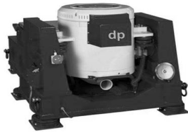
Figure 8-31 - Shaker to be used to excite natural frequencies
