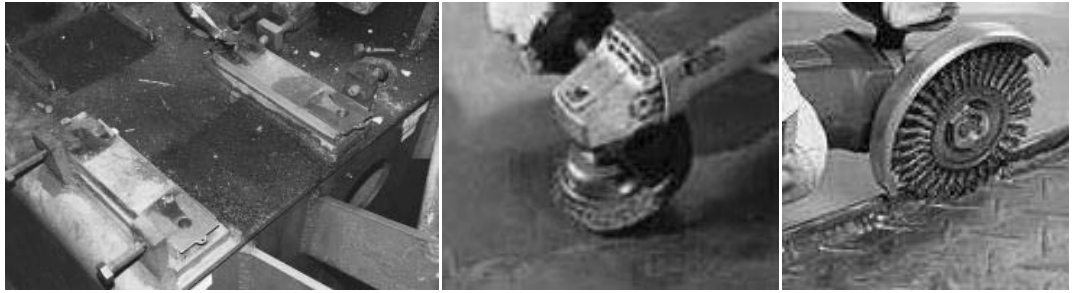
Figure 12-31 Remove dirt, grit, burrs and other debris
