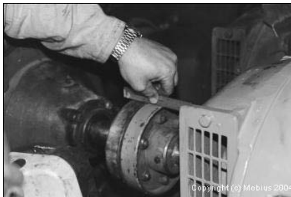
Figure 12-10 Machines will likely be misaligned if precision alignment was not performed
