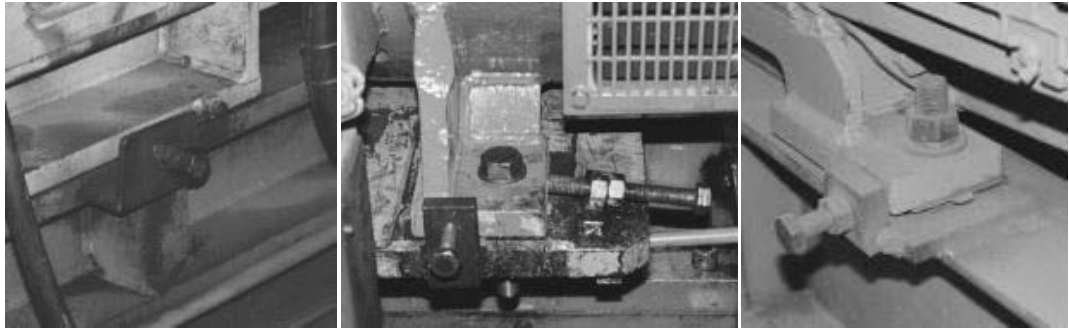
Figure 12-63 Jacking bolts for lateral movement
