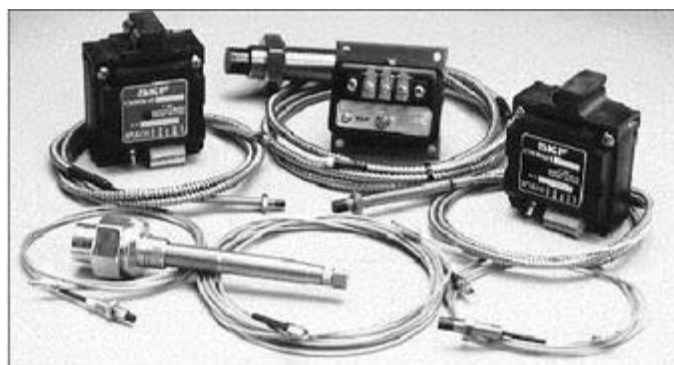
Figure 6-16 - Eddy current probes have 3 components: the probe, a driver, and the cable between them.
