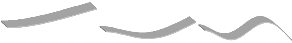
Figure 8-32 - The three mode shapes of the cantilevered bar
