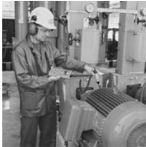
Figure 23-19 Direct Contact probe is useful for detecting bearing problems
