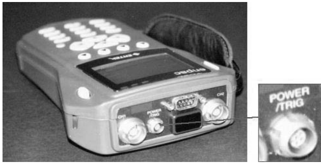
Figure 6-93 - the tach input may be labeled trigger or phase.
