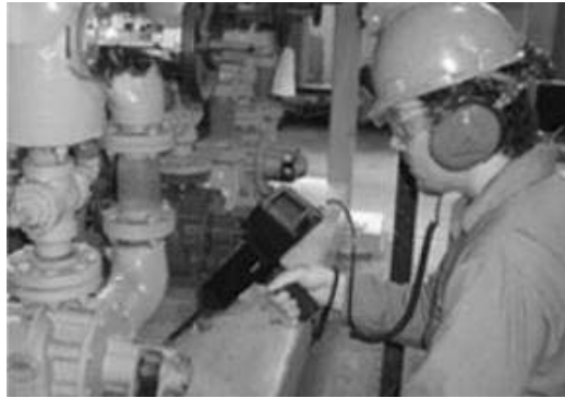
Figure 23-13 A Direct Contact probe uses a “stinger” to capture the sounds
