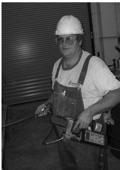
Figure 14-10 an ultrasound device integrated into a grease gun
