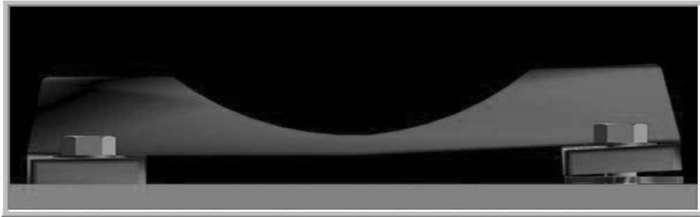
Figure 11-21 - Soft foot condition can cause 1x, 2x, and 3x peaks as well as twice line frequency.
